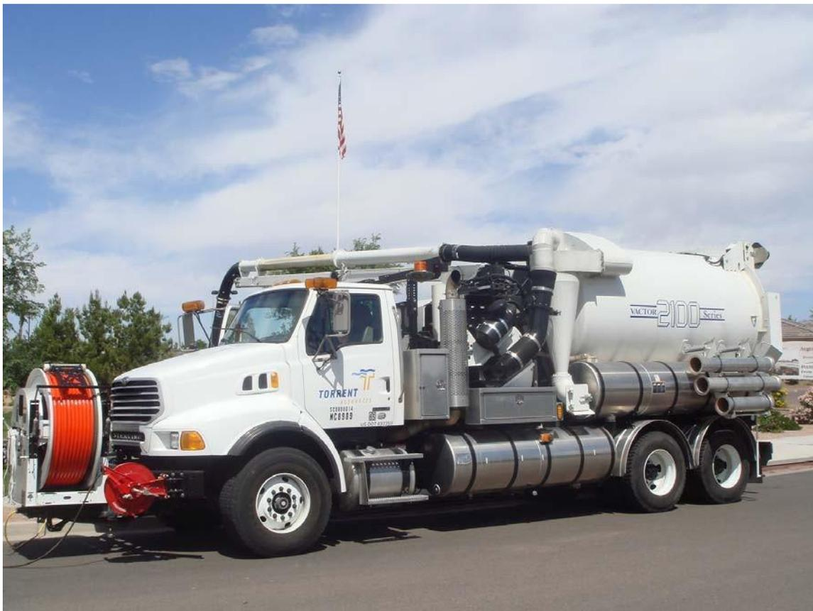
Typical Hydrovector Truck used for Drywell Maintenance
