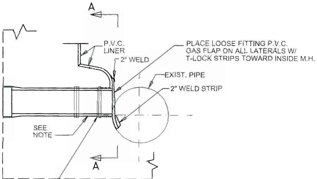
WRAP P.V.C. LINER AROUND V.C.P. AND SECURE WITH STEEL BAND RING WITH TAKE UP BOLT.
