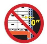
*Note:* Flue space is measured as the distance between the loads, not the distance between the racks. A flue space's net width is a measure of its gross width minus any horizontal obstructions, such as rack uprights, located within the flue space. In other words, a rack upright (typically 3 in. wide) is not considered a flue space, due to the cross bracing used.
